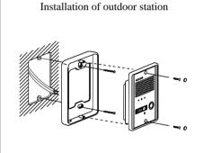
After attaching the body supporter with 2screws, put the indoorstation into the grooves of body supporter, and then fix it with screws.
